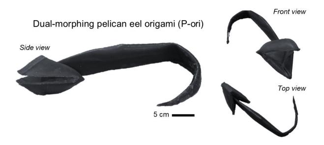
The dual-morphing pelican eel origami robot. Credit: Kim et al., Sci. Robot. 4, eaay3493 (2019)
