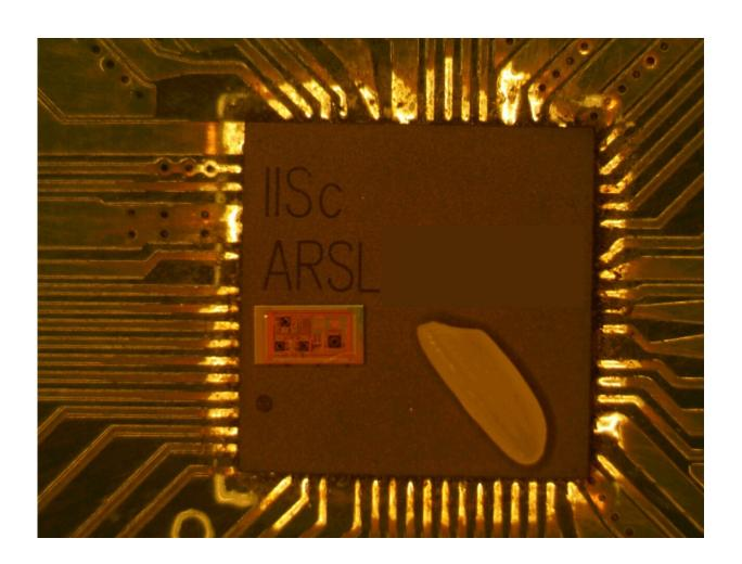
A photomicrograph of the TWR radar-on-chip compared to a grain of rice. Credit: ARSL, IISc
