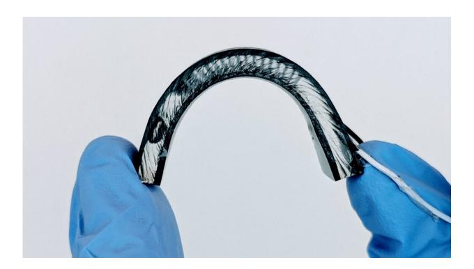
NC State's improved theromoelectric generator demonstrates efficiency and flexibility. Credit: Mehmet Ozturk, NC State University.
