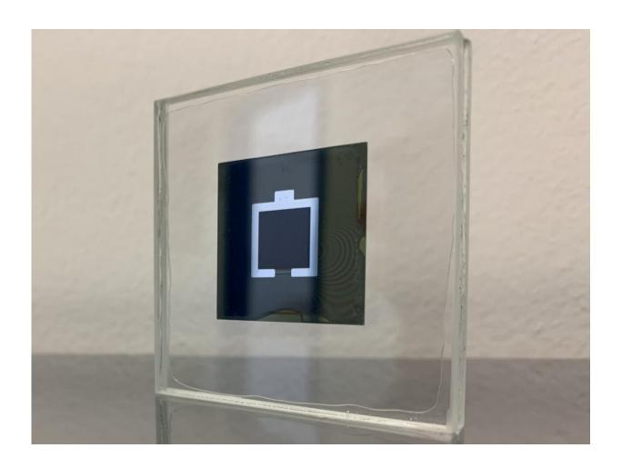
The tandem solar cell was realized on a typical laboratory scale of one square centimeter. However, scaling up is possible. Credit: Eike Köhnen/HZB
