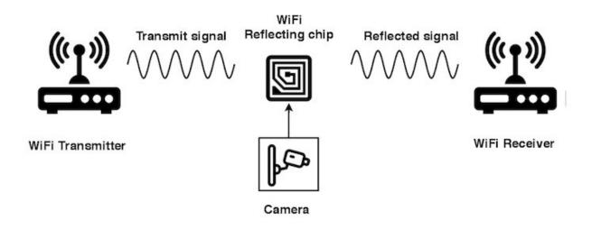
Illustration of the backscattering process. Credit: University of California - San Diego
