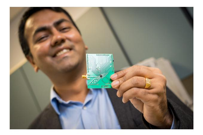
UC San Diego electrical and computer engineering professor Dinesh Bharadia holds a PCB onto which the Wi-Fi radio is mounted (component underneath the black blob). Credit: University of California - San Diego
