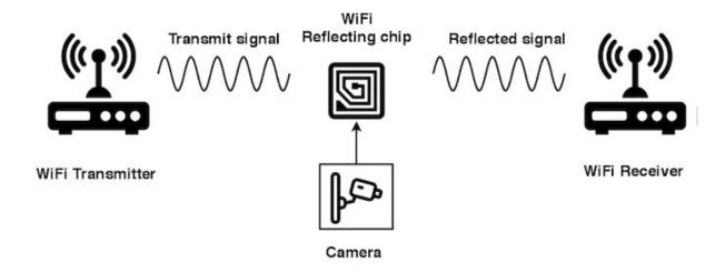
Illustration of the backscattering process. Credit: University of California - San Diego
