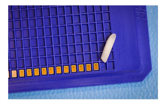
A set of ultra-low power Wi-Fi radios integrated in small chips, each measuring 1.5 square millimeters in area (grain of rice shown for scale). Credit: David Baillot/UC San Diego Jacobs School of Engineering.
