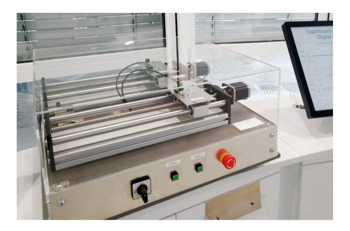
Demonstrator set-up with two recirculating ball spindles. Credit: Fraunhofer IPK
