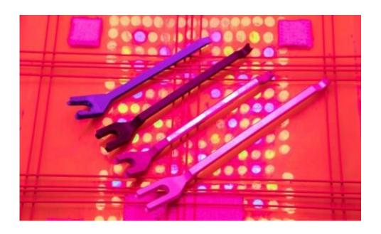
NASA use 3D-printed tools too: this shows the evolution of their 'bungee' tool as it went from a simple, 3D-printed object to an increasingly refined tool used in the Veggie plant chamber aboard the International Space Station. Credit: NASA
