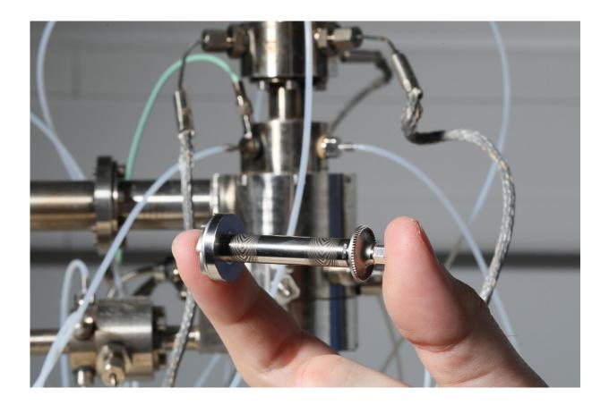
The shaft with steam-lubricated bearings developed at EPFL. Credit: EPFL 2020
