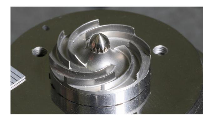
Off-gas recirculation fan developed at EPFL's Laboratory for Applied Mechanical Design (LAMD). Credit: EPFL
