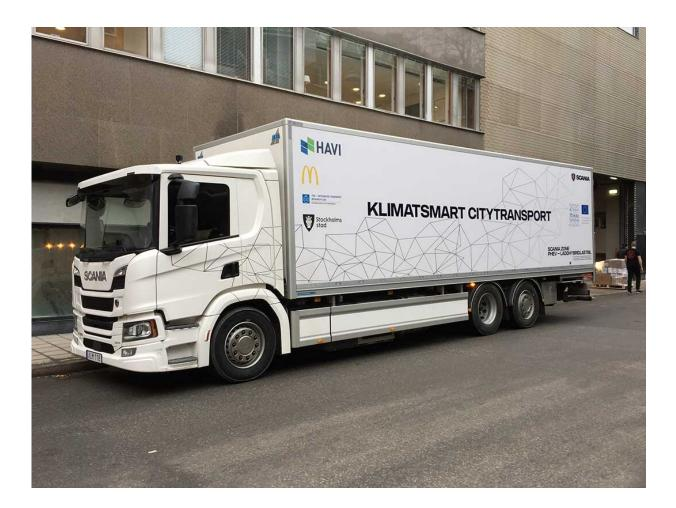
The hybrid truck trialled in Stockholm, Sweden, runs on hydrotreated vegetable oil outside the city and electricity in the centre, and delivered to six restaurants on a single charge. Credit: Paul Fenton
