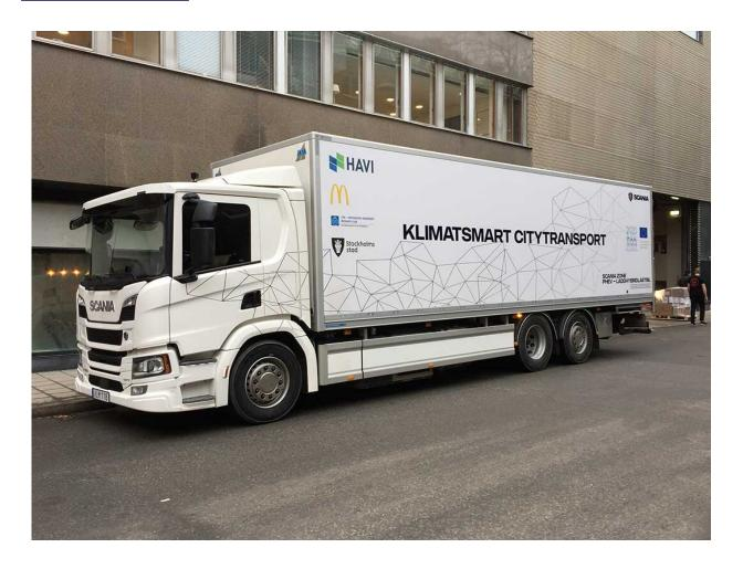
The hybrid truck trialled in Stockholm, Sweden, runs on hydrotreated vegetable oil outside the city and electricity in the centre, and delivered to six restaurants on a single charge. Credit: Paul Fenton
