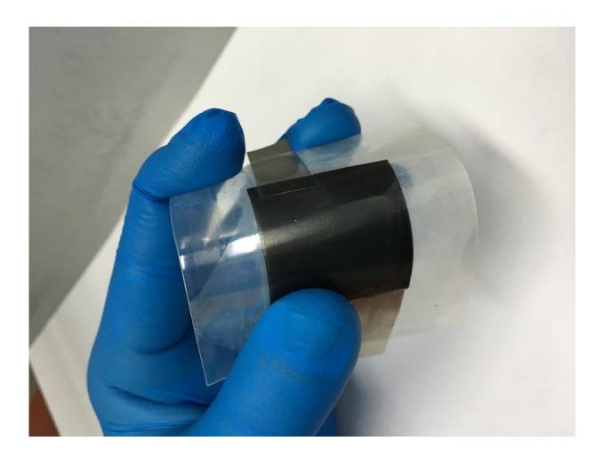
A new bendable supercapacitor made from graphene, which charges quickly and safely stores a record-high level of energy for use over a long period. Credit: Dr Zhuangnan Li (UCL)
