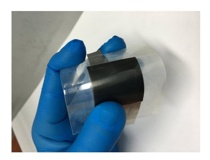
A new bendable supercapacitor made from graphene, which charges quickly and safely stores a record-high level of energy for use over a long period. Credit: Dr Zhuangnan Li (UCL)
