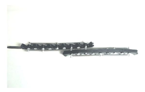
With a small push, these deployable structures can go from flat to curved. Credit: Bertoldi Lab/Harvard SEAS
