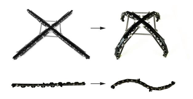
Deployable structures transition from flat to domed and straight to curved with a small push. Credit: Bertoldi Lab/Havard SEAS
