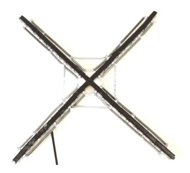
This deployable structure uses the same principles as falling dominos to transition from flat to domed. Credit: Bertoldi Lab/Harvard SEAS
