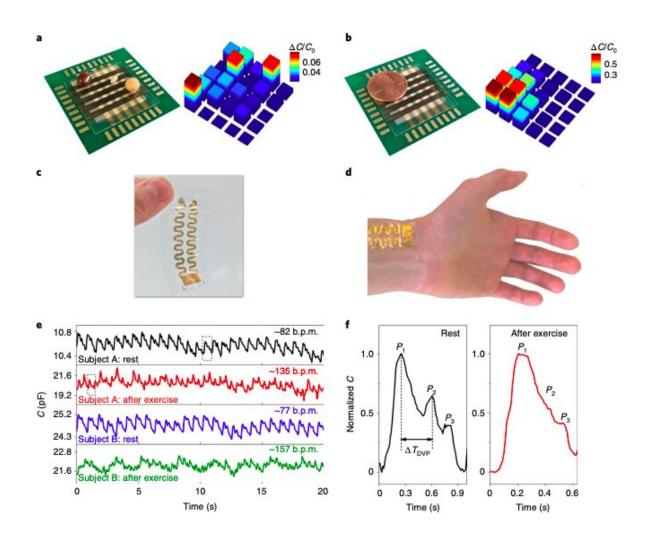
Flexible CMAG capacitor-based pressure sensors for static pressure mapping and real-time pulse wave monitoring of the radial artery. a) Photograph of a  $5 \times 5$ -pixel array with grains of rice, soybean and red bean weighing ~20, 158 and 219 mg, respectively (left), and the corresponding distribution of the normalized
