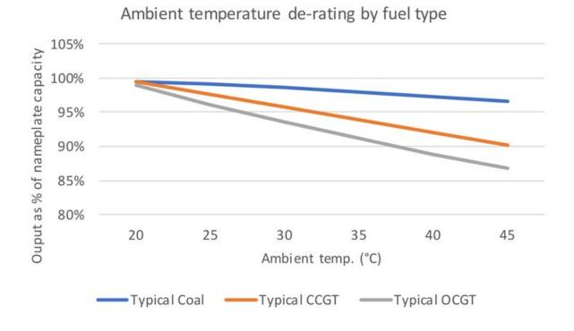
This graph shows how the efficiency falls for coal-power turbines, combinedcycle gas turbines and open-cycle gas turbines falls as the temperature increases. Credit: Australian Energy Market Operator
