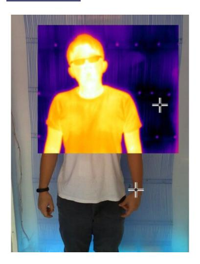
As shown by a thermal camera, the person is cool when standing in front of a radiant cooling system. Credit: Eric Teitelbaum
