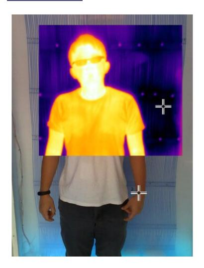
As shown by a thermal camera, the person is cool when standing in front of a radiant cooling system. Credit: Eric Teitelbaum
