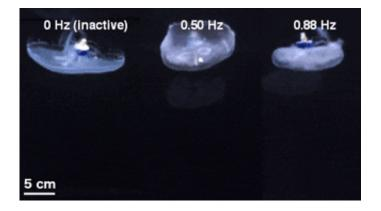
A comparison of bell geometries for unstimulated swimming with an inactive swim controller embedded (left) and externally controlled swimming at 0.50 Hz (middle) and 0.88 Hz (right). Credit: Science Advances, doi: 10.1126/sciadv.aaz3194
