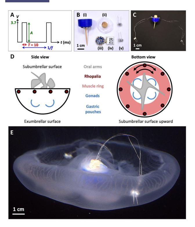
A. aurita swim controller design. (A) Square wave signal generated by the swim controller with an amplitude (A) of 3.7 V and a pulse width (T) of 10 ms, set at frequencies (f) of 0.25, 0.38, 0.50, 0.62, 0.75, 0.88, and 1.00 Hz. (B) Swim controller components. Housing includes (i) a polypropylene cap with a wooden
