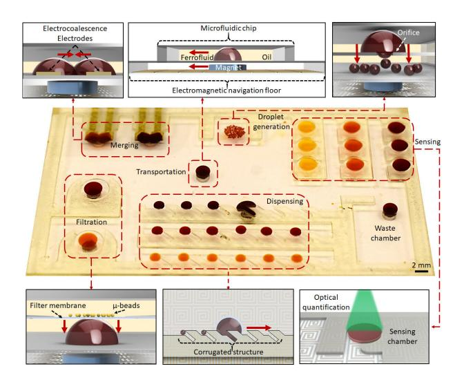
Overview of microfluidic system concept and mechanism. Credit: Yu et al., Sci. Robot. 5, eaba4411 (2020)
