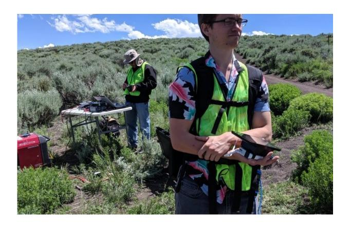
NIST electronics engineer Hien Nguyen sets up test equipment to make cellular signal measurements, while NIST computer science intern Josh Hamel prepares to take a walk to measure signal strength and coverage characteristics. Credit: National Institute of Standards and Technology
