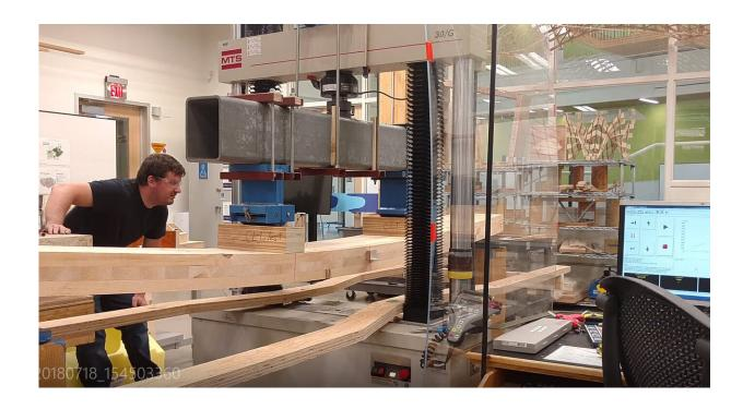
Panels of CLT were placed into a strength-testing machine at the UMass Wood Mechanics Lab, where a giant steel arm put thousands of pounds of pressure on the engineered wood until it broke. Credit: Peggi Clouston/UMass Amherst
