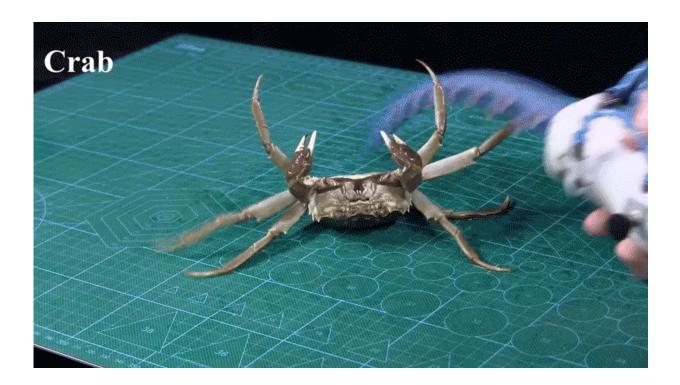
The soft robot is controlled with two valves, one to apply pressure for bending the arm and one for a vacuum that engages the suckers. By changing the pressure and vacuum, the arm can attach to any object, wrap around it, carry it, and release it. Credit: the Bertoldi Lab/Harvard SEAS
