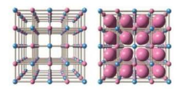
Crystal structure of cobalt Prussian blue analog LixCo[Fe(CN)6]y. The left figure shows the time of complete charge, and the right figure shows the time of complete discharge. Large red circle, small blue circle, small red circle indicate lithium ion, cobalt ion, iron ion, respectively. Credit: University of Tsukuba
