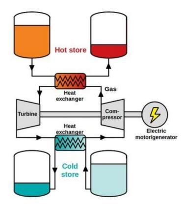
The conversion of electricity to heat happens in the central circuit, then stored in hot and cold tanks. Credit: Pau Farres Antunez, Author provided
