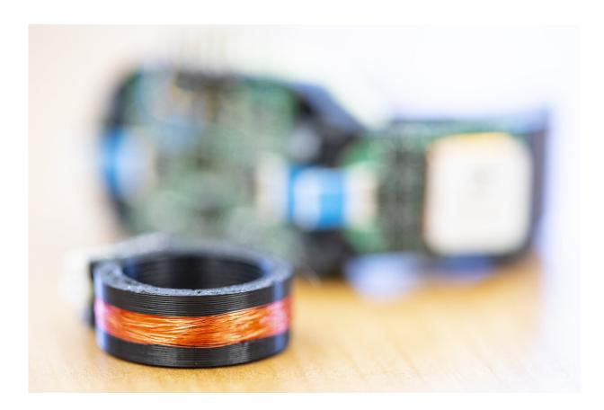
Researchers at the University of Washington have created AuraRing, a ring (foreground) and wristband (background) combination that can detect the precise location of someone's index finger -- and continuously track hand movements. Credit: Dennis Wise/University of Washington
