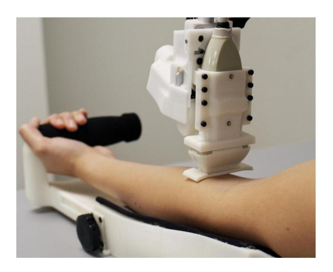
A prototype of an automated blood drawing and testing device. Credit: Unnati Chauhan
