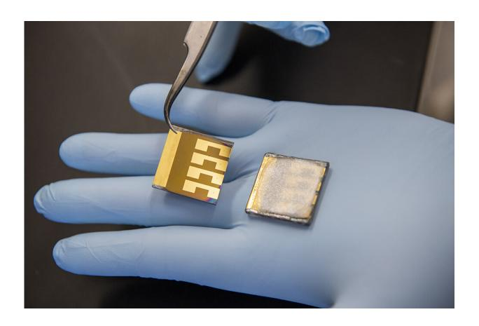
Two laboratory solar cell samples, one (right) with a protective lead-absorbing film applied to the backside. Credit: Northern Illinois University
