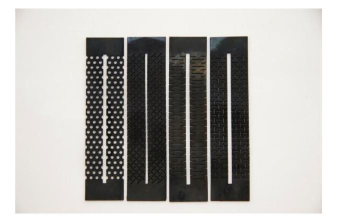
The researchers' soft sensors are conductive silicone sheets cut into kirigami patterns. They have "piezoresistive" properties, meaning they change in electrical resistance when strained. As the sensor deforms in response to the robotic arm's stretching and compressing, its electrical resistance is converted to an output voltage that's then used as a signal correlating to that movement. Credit: Ryan L. Truby, MIT CSAIL
