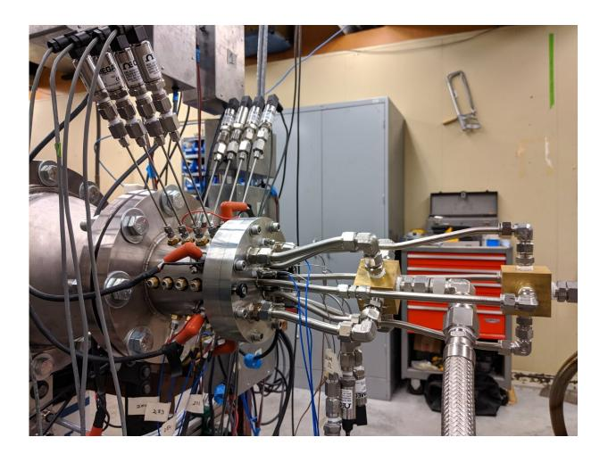
The researchers first developed an experimental rotating detonation engine (shown here) where they could control different parameters, such as the size of the gap between the cylinders. The feed lines (right) direct the propellant flow into the engine. On the inside, there is another cylinder concentric to the outside piece. Sensors sticking out of the top of the engine (left) measure pressure along the length of the cylinder. The camera would be on the left-hand side, looking
