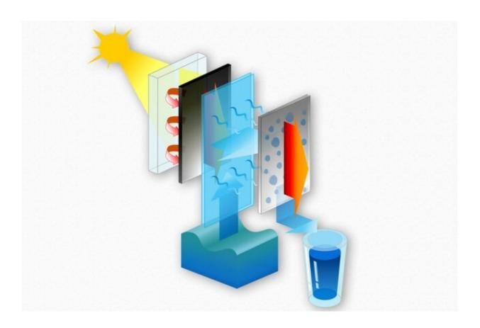
Diagram illustrates the basic structure of the proposed desalination system. Sunlight passes through a transparent insulating layer at left, to heat up a black heat-absorbing material, which transfers the heat to a layer of wicking material (shown in blue), where it evaporates and then condenses on a surface (gray) and then drips off to be collected as fresh, potable water. Credit: Massachusetts
