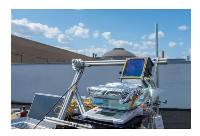
Tests on an MIT building rooftop showed that a simple proof-of-concept desalination device could produce clean, drinkable water at a rate equivalent to more than 1.5 gallons per hour for each square meter of solar collecting area. Credit: Massachusetts Institute of Technology
