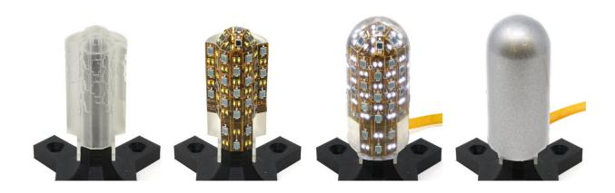
Tactile fingers progressing through its manufacturing stages: 3D-printed skeleton, flexible circuit board, transparent silicone layer, and reflective skin. Credit: Pedro Piacenza / Columbia Engineering
