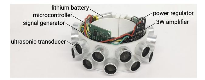
Figure 3. Our prototype is a self-contained wearable comprised of ultrasonic transducers, a signal generator, a microcontroller, a battery, a voltage regulator and a 3W amplifier. Credit: Yuxin Chen et al.
