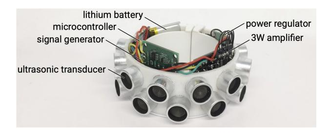
Figure 3. Our prototype is a self-contained wearable comprised of ultrasonic transducers, a signal generator, a microcontroller, a battery, a voltage regulator and a 3W amplifier. Credit: Yuxin Chen et al.
