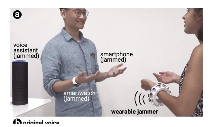
Figure 1. (a) We engineered a wearable ultrasound jammer that can prevent surrounding microphones from eavesdropping on a conversation. (b) This is the actual speech that the conversation partner hears, since our jammer does not disrupt human hearing. However, (c) is the transcript of what a state-of-the-art speech recognizer makes out of the jammed conversation. Credit: Yuxin Chen et al.
