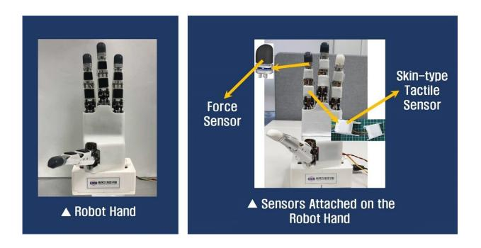
Tactile Sensor-integrated Robot Hand. Credit: Korea Institute of Machinery and Materials (KIMM)
