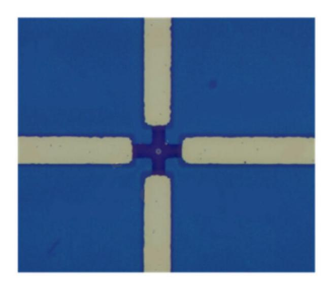
An optical image of the device structure with 4 micrometer pillar diameter. Credit: Northwestern University/University of Messina, Italy
