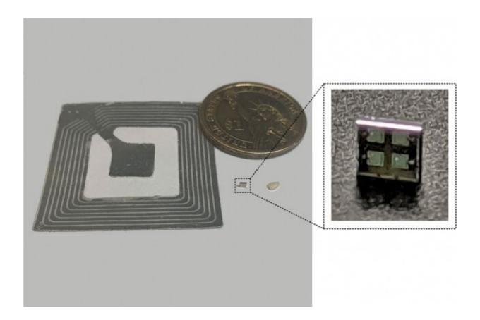
Even though it's the size of a sesame seed, the ID tag (zoomed in, right) can send wireless communications at greater reader distances than much larger RFID tags (left) and can run cryptographic algorithms to help secure nearly any product in the supply chain. Credit: Massachusetts Institute of Technology
