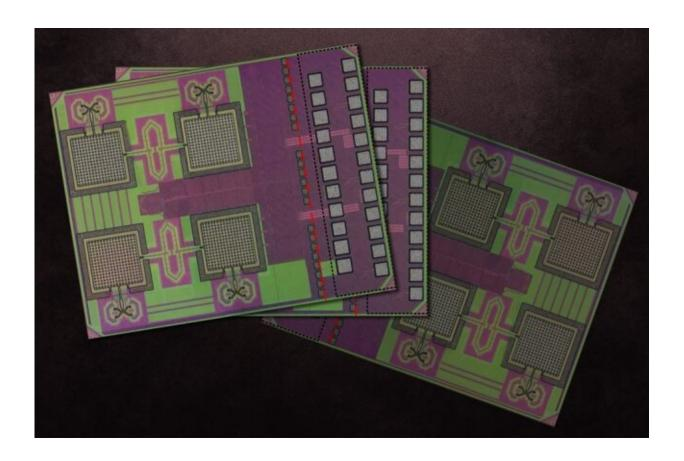
MIT researchers' millimeter-sized ID chip integrates a cryptographic processor, an antenna array that transmits data in the high terahertz range, and photovoltaic diodes for power. Credit: MIT News
