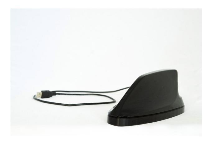
Teaching cars to hear: a modified roof fin for testing acoustic sensors for the capture of external noise. Credit: Fraunhofer IDMT/Hannes Kalter
