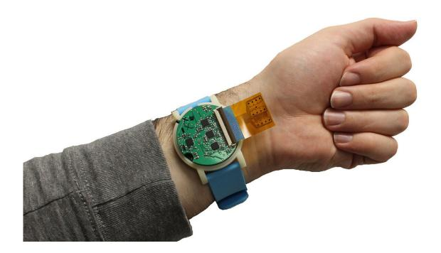
The metabolite monitoring device, shown here, is the size of a wristwatch. The sensor strip, which sticks out in this photo, can be tucked back, lying between the device and the user's skin. Credit: Murat Yokus, NC State University
