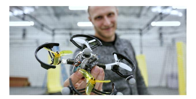
A robust drone controller, trained using reinforcement learning algorithms developed by USC researchers allows drones to withstand harsh treatment, including being thrown and pushed. Credit: Haotian Mai
