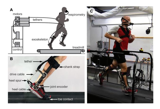
Experimental setup and ankle exoskeleton design. The ankle exoskeleton
