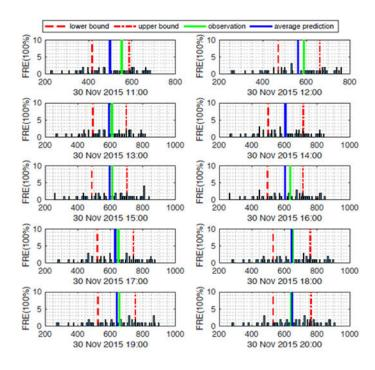
Prediction uncertainty analysis. The green line is the actual PM2.5 levels measured from a sensor. The blue line is the system's PM2.5 prediction. The red lines outline the probability range the system believes the levels will fall within. Credit: Loughborough University
