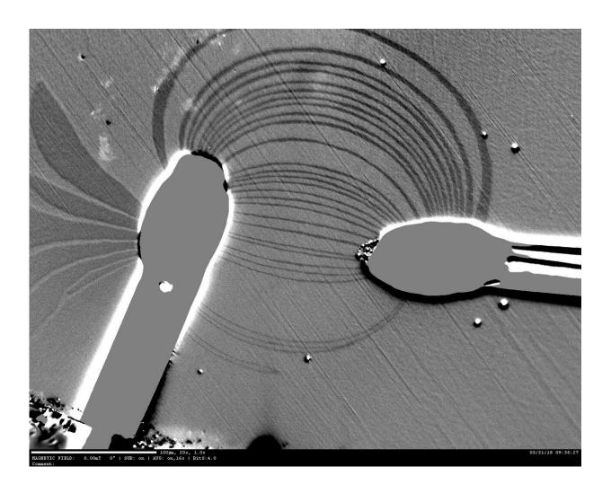
The flow of an electric current between two electrodes on a magnetic thin film are imaged by measuring the strip domains. Credit: KAUST
