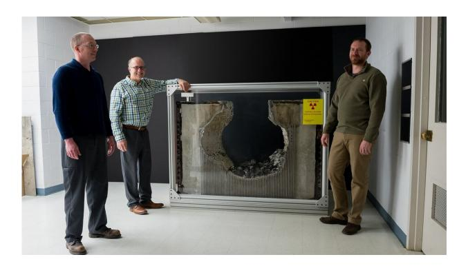
Nathan Bremer, Mitch Farmer (center) and Jeremy Licht (right) highlight a piece of concrete eroded in tests by corium — the lava-like material formed when uranium fuel rods in the reactor core melt, along with their protective metal cladding. The team's tests helped nuclear plant operators avoid \$1 billion in expenses. Not shown: Stephen Lomperski and Dennis Kilsdonk. Credit: Argonne National Laboratory
