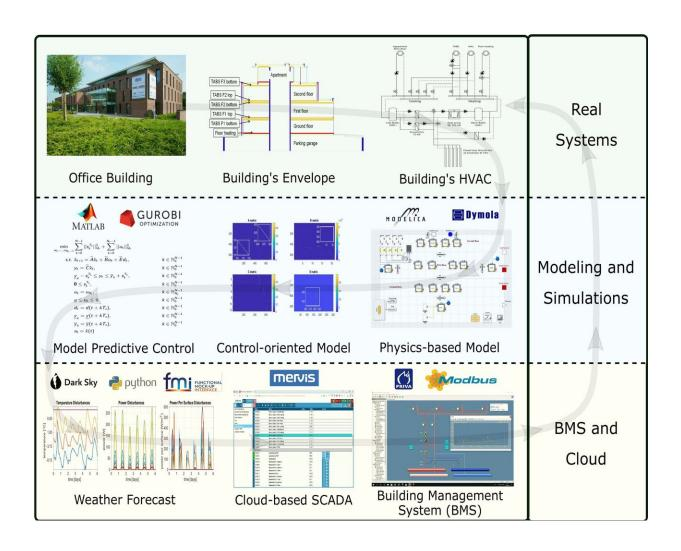
This detailed graphic conveys the research team's methodology, which draws upon deep learning methods to help transform relevant simulation data into strategies for real-time control of building operations. The building and its real systems, combined with modeling and simulations as well as other data, influence the building management system, leading to enhanced control of building operations. Credit: Pacific Northwest National Laboratory
