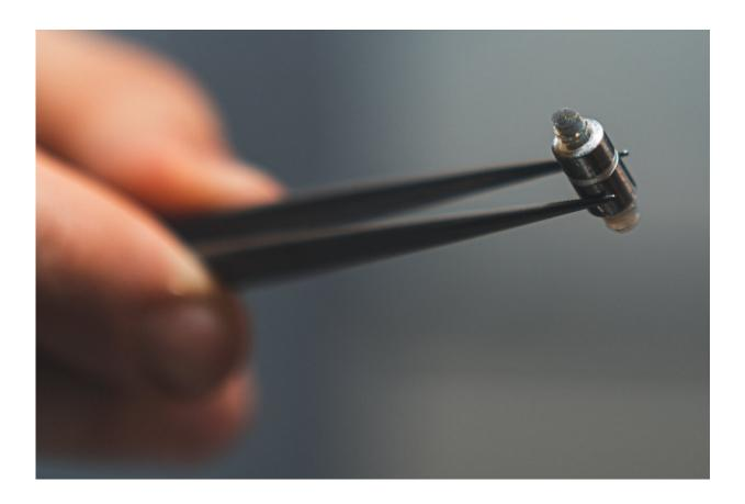
A close up of the microwire array. With a silicon chip attached to the top and the wires at the bottom gently inserted into the brain, this device can help researchers take a movie of neural activity. Credit: Andrew Brodhead
