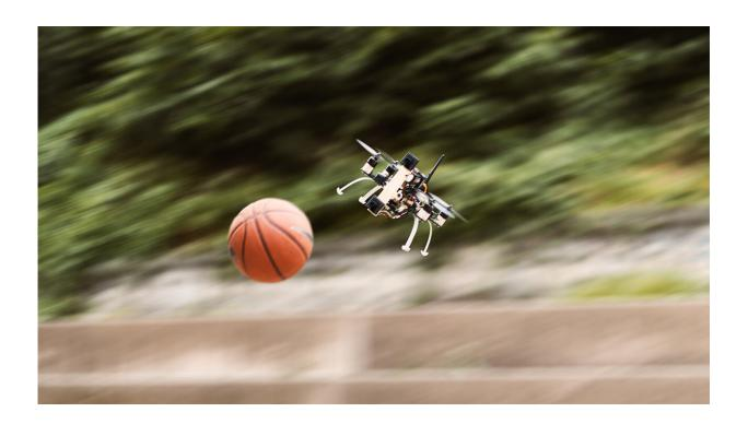
The drone is able to successfully dodge - even if the ball is approaching it from a distance of three meters at 10 m/s. Credit: UZH
