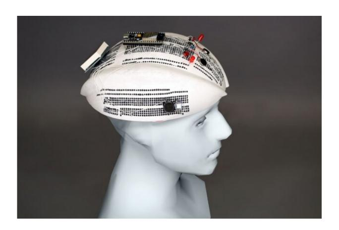
CurveBoards are 3D breadboards — which are commonly used to prototype circuits — that can be designed by custom software, 3D printed, and directly integrated into the surface of physical objects, such as smart watches, bracelets, helmets, headphones, and even flexible electronics. CurveBoards can give designers an additional prototyping technique to better evaluate how circuits will look and feel on physical products that users interact with. Credit: Dishita Turakhia and Junyi Zhy
