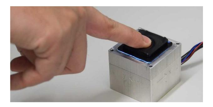
The tactile sensor prototype. Credit: ETH Zurich
