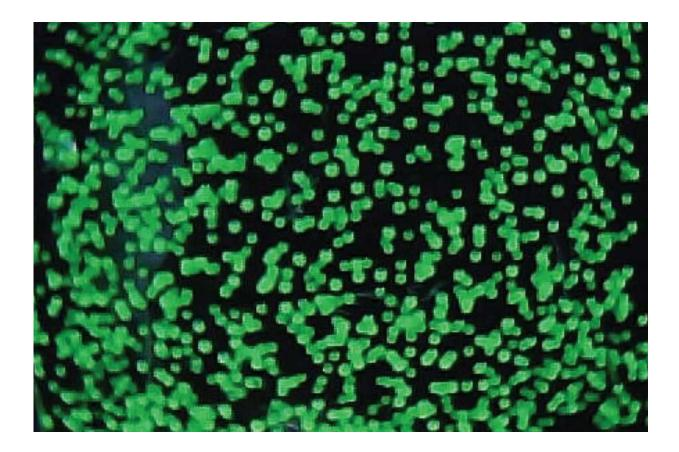
Microbeads on the underside of the silicone skin. A camera registers how they move when a force acts upon them. Credit: ETH Zurich
