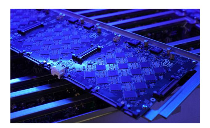
A closer look shows one of the rows within Intel's latest neuromorphic research system, Pohoiki Springs. The system, unveiled in March 2020, is made up of eight of these rows, with each containing three 32-chip Intel Nahuku boards, for a total of 768 Loihi chips. The ninth row is made up of Arria10 FPGA boards.
