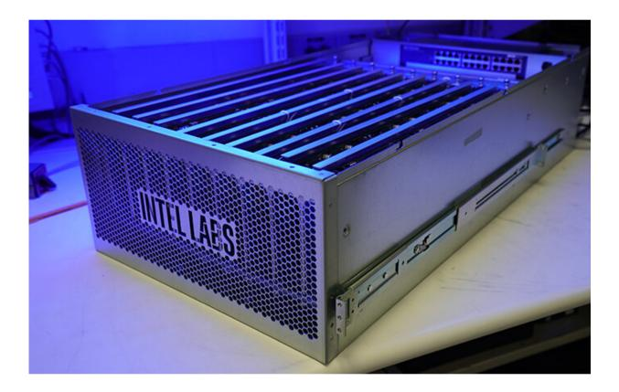
Pohoiki Springs, a data center rack-mounted system unveiled in March 2020, is Intel's largest neuromorphic computing system developed to date. It integrates 768 Loihi neuromorphic research chips inside a chassis the size of five standard servers. Credit: Intel Corporation
