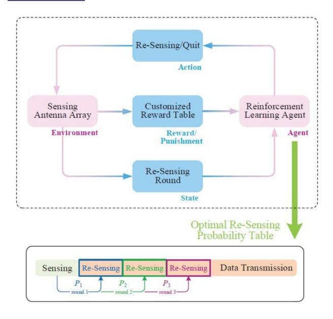
Reinforcement-learning-driven automatic repeat sensing mechanism. Credit: SARI
