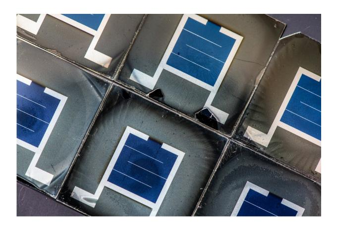
Perovskite/silicon tandem solar cells are contenders for the next-generation photovoltaic technology, with the potential to deliver module efficiency gains at minimal cost. Credit: Dennis Schroeder / NREL
