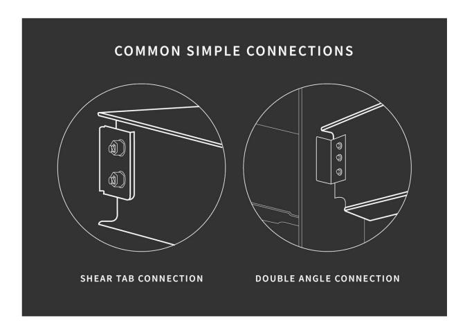
The shear tab connection (left) is a single flat plate welded to the support column and bolted onto one side of the steel beam. The double angle connection (right) is composed of two L-shaped plates, or angle legs, welded to the support column and bolted onto both sides of the steel beam. In this study, the double angle-connected beams endured greater deformations and temperatures before failing. Credit: B. Hayes/NIST
