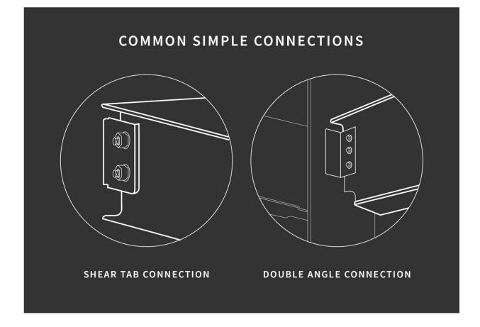
The shear tab connection (left) is a single flat plate welded to the support column and bolted onto one side of the steel beam. The double angle connection (right) is composed of two L-shaped plates, or angle legs, welded to the support column and bolted onto both sides of the steel beam. In this study, the double angleconnected beams endured greater deformations and temperatures before failing. Credit: B. Hayes/NIST
