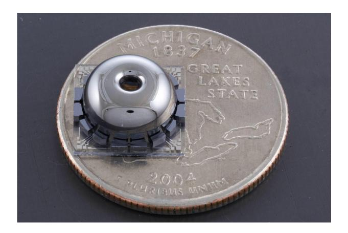
The new resonator and electrodes, on a quarter for scale. The resonator is almost perfectly symmetrical, made of nearly-pure glass. This enables it to vibrate for long periods, similar to the ringing of a wine glass. Credit: Najafi Group, University of Michigan
