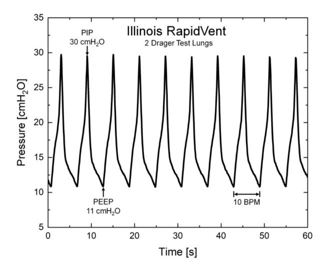
Pressure controlled cycling of the prototype emergency ventilator connected to two Drager test lungs powered by air at 50 psi, showing consistent peak inspiratory pressure (PIP) and positive end expiratory pressure (PEEP). Credit: Illinois RapidVent
